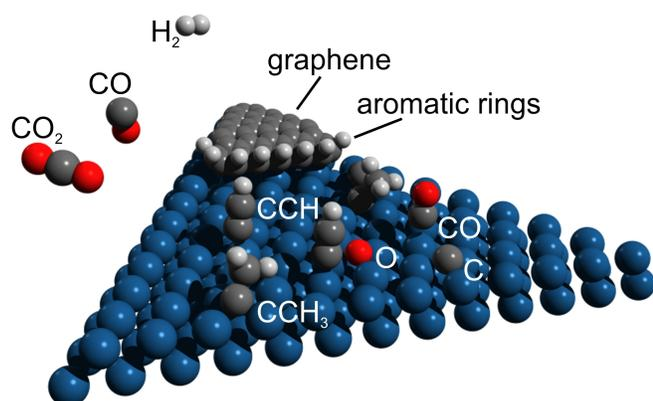
**Figure 1.** Cartoon summary of the stable adsorbed species identified at the Ir(111) surface upon hydrogenation of CO and CO<sub>2</sub> at NAP conditions.
